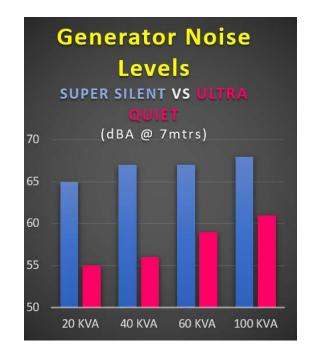
Featuring a specifically designed sound attenuated canopy, our Ultra Quiet sets run at around 10 decibels quieter than a standard Super Silent Generator, making them the ideal choice for noise sensitive applications.
